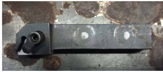
Figure 2. Toolholder Type MTGNR2020K16
