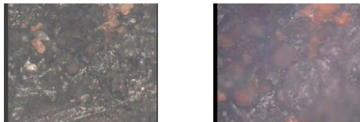
(a) (b) Fig. 6 (a) Microstructure of ST60 Steel magnification of 100x after corrosion test in 0.1 M NaCl (b) Microstructure of ST60 Steel magnification of 200x after corrosion test in 0.1 M NaCl
