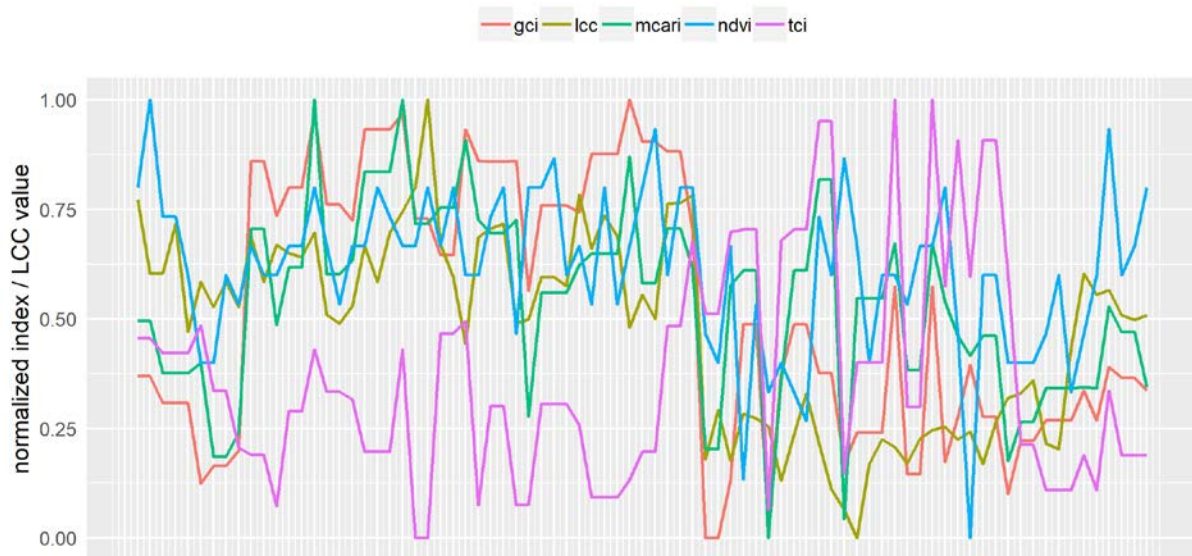
Figure 1. Trend of evaluated spectral indices derived from Sentinel-2 imagery and normalized LCC among the number of 81 sampling points.
