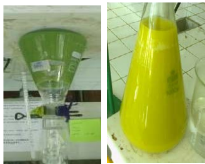
Figure 2. Zeolite Color Changes During Activation
